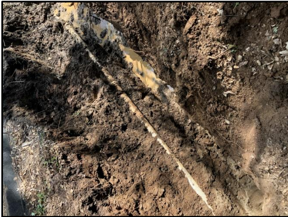
Broken Sch 40 4" PVC Split 20' due to deflection in the pipe and poor installation
