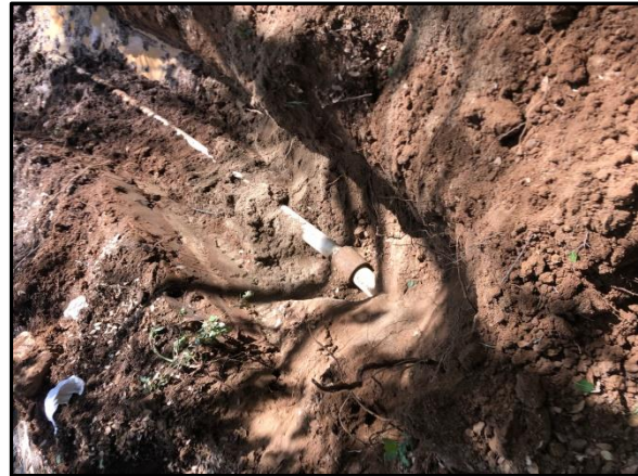
Broken Sch 40 4" PVC Split 20' due to deflection in the pipe and poor installation
