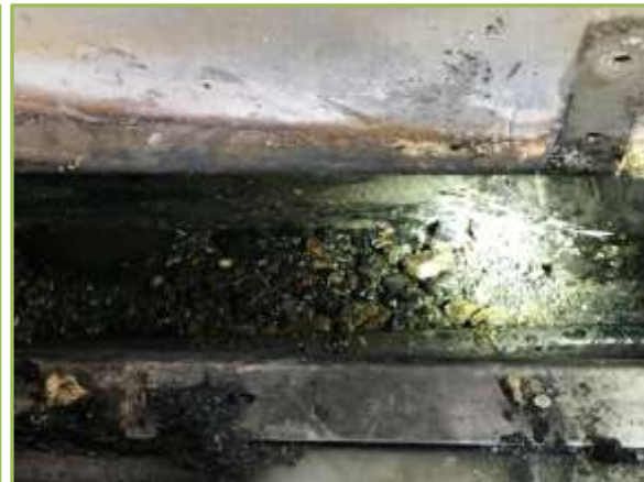
Sand and Debris that plugged the inlet to roto drum #2
