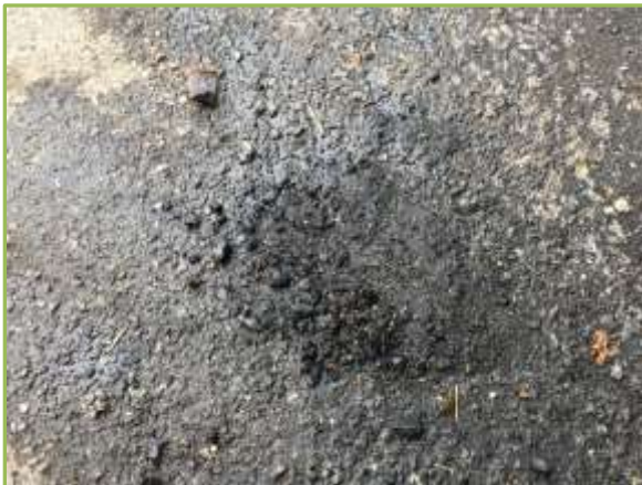
Sand and Debris that plugged the inlet to roto drum #2
