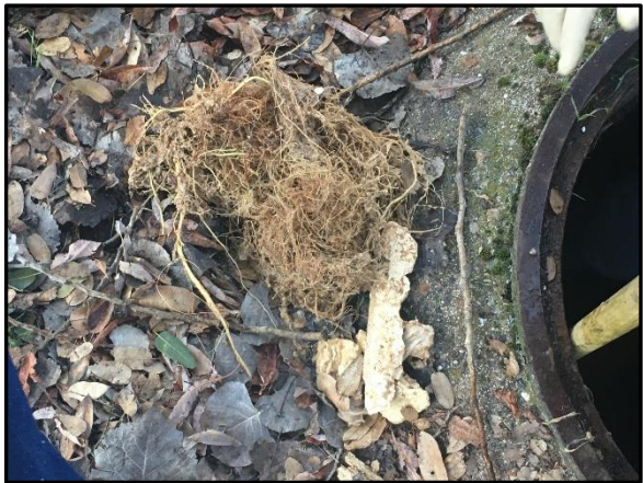
Root ball and grease broken lose from Hydro Flushing left Root ball and grease removed right
