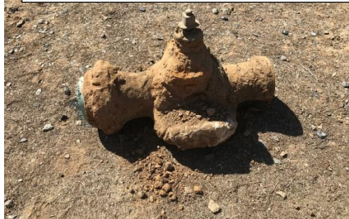
Old valve Dated 1979 was cut out and replaced with new section. Valve was stuck in the open position
