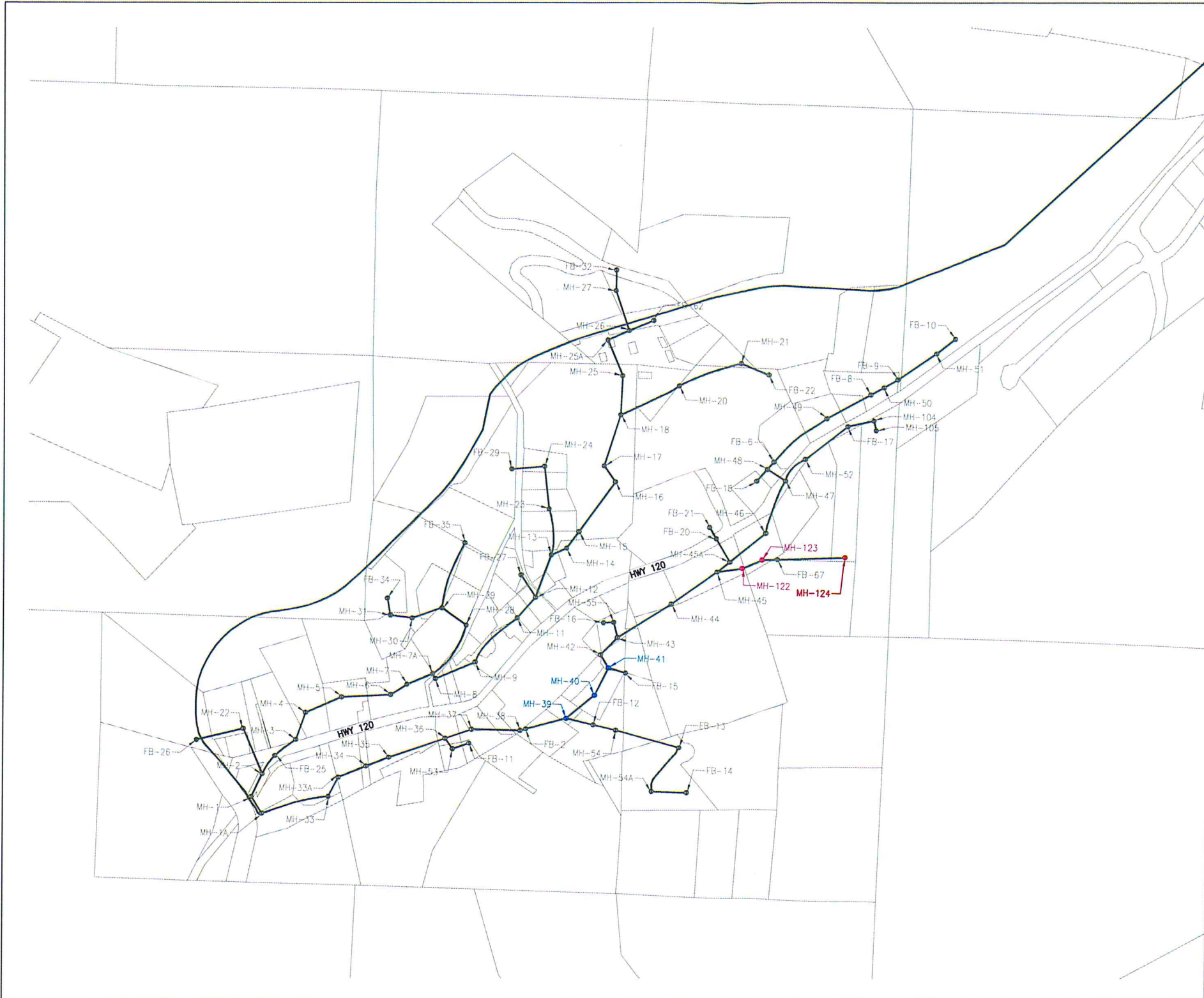
FIGURE 4-3 ALTERNATIVES II & III BIG OAK FLAT MANHOLE IMPROVEMENTS
